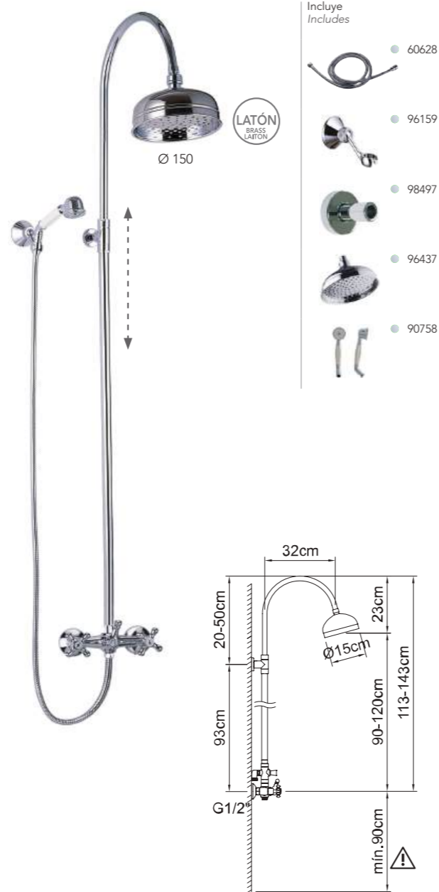
Conjunto de ducha bimando con barra extensible y soporte articulado. Two-handed shower set with extendable bar and articulated support.
